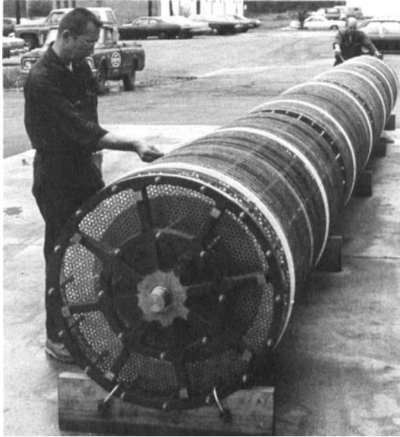
FIGURE 4. Plate stack showing end spider plate.
